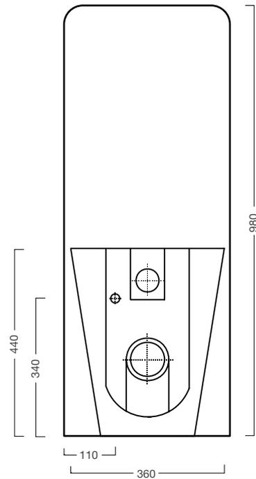
\* Monolith includes a double flow anticondensation plastic cistern system
